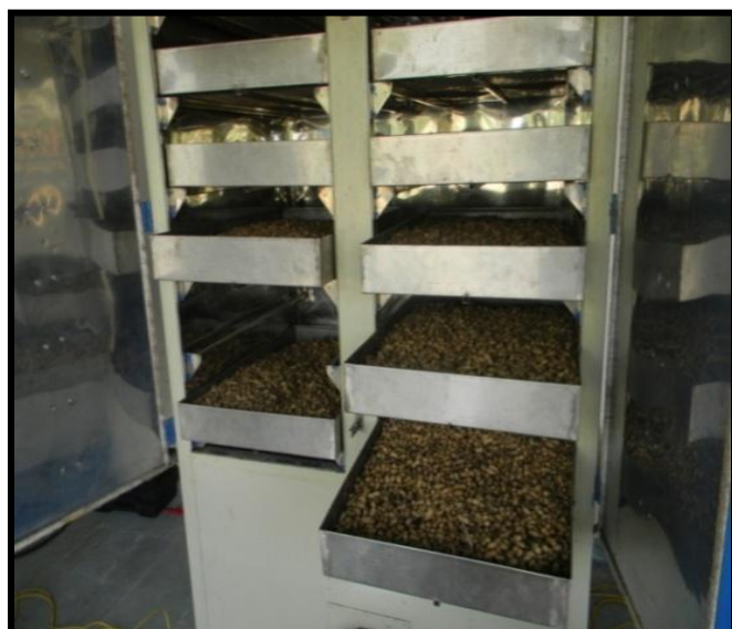
Plate 3: Drying of groundnut pods using solar dryer
